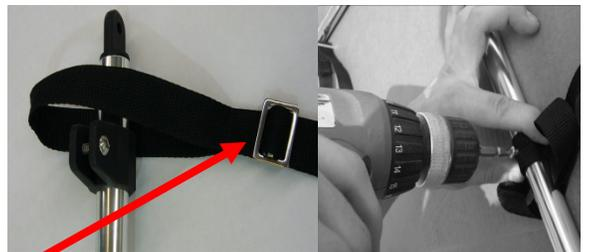
Step 4. Pass looped end of each hold-down strap over each end of the long (A-bow) and medium (B-bow). Use a #8 x 1/2" screw to fasten strap to bow frame at each pre-drilled hole position as shown. Position strap over hole and insert screw, with finish washer, through center of strap and into pre-drilled hole. Be sure the adjuster buckle is facing out.
