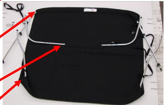
Step 6. Pass the medium (B-bow) assembly through the sleeve at the front of the top. Be sure screws for hold-down straps are facing down.
