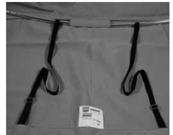
(Adjuster straps will be used to achieve desired crown on Bimini Top after installation on boat. See enlargement on page 6.)
