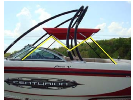
Placement of the hold-down straps should form the letter "M". Straps should form a 45 to 90 degree angle with each bow.
