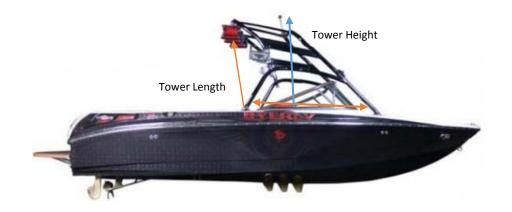
Fits boats with the tower mounted over the windshield with the top of the tower not to exceed 24" behind the wing of the windshield. Max tower height from top of gunnel: 68".
