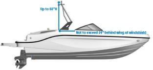
Fits boats with the tower mounted over the windshield with the top of the tower not to exceed 24" behind the wing of the windshield. Max tower height from gunwale: 68". See diagram.
